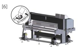
Tighten the handle on the origin side of the rear roll unit.
