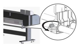
Twist the knob bolt on the both side of the media holders anticlockwise to
