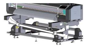
Attach a paper core to the origin side of the front roll unit.
