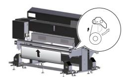
Hold the leading edge of a roll media with your one hand and push the rear tension roller as far as it will go to unwind roll media.
