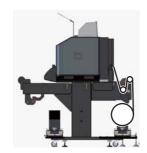
The media should be loaded to the roller as shown in the illustration when seen from the side.
