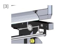
Attach the weight (1 piece) to the weight mount board R with a M4×16 screw.
