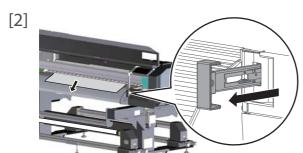
Laise the pressure rollers and pull the media from the media feed slot.
