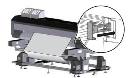
Check that the pressure rollers are locked (lowered).
