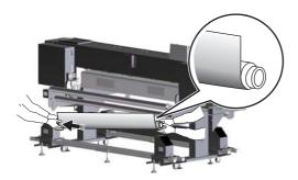
Attach the roll media to the origin side of the rear roll unit.
