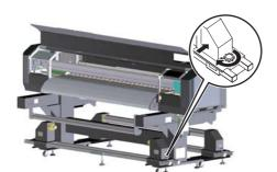
Tighten the handle on the origin side of the front roll unit.
