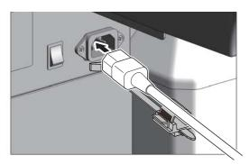
Connect the power cord of the heavy-duty take-up unit to the printer.
