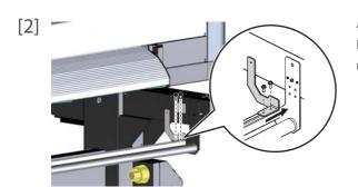
Attach the weight mount board R to the origin side of the front tension roller. Insert and tighten the two M4×12 screws in the post-assembly insertion short
