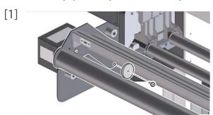
Attach the weight (1 piece) to the origin side of the rear tension roller with a M4×16 screw.
