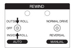
Go to the front of the printer and make sure the AUTO switch for the Take-Up Unit is OFF.
