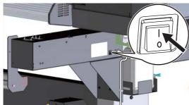
Press the power button to turn the power ON.
