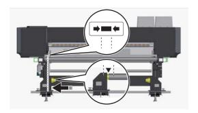
Move the origin side of the rear roll unit to the position that the left end of the roll media ( ▼ in the left illustration) is aligned within the mark on the label applied to the balance frame on the rear tension roller (within the range between two dotted lines shown left).
