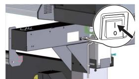
Press the power button to turn the power ON.
