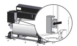
Lower the pressure rollers to temporarily hold down the roll media.
