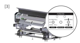
Turn the MANUAL switch on the feed unit according to the printing side of your roll media to pull the roll media out about 1 m.
