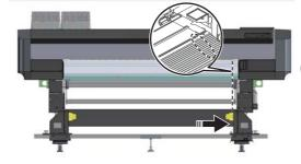
• Align the origin side of the front roll unit with the media registration guide holes on the printer (holes on the media guide).
