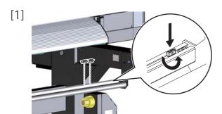
Attach two post-assembly insertion nuts to the balance frame on the front tension roller.
