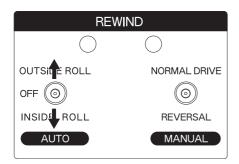
Set the AUTO switch according to the media rolling direction.
