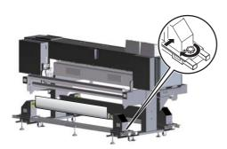
Tighten the handle on the non-origin side of the rear roll unit.
