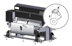
Pass it under the roller in the back, then up to pass through the rear tension roller as shown.
