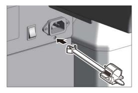
Attach the cord clamp to the front tension unit (on the origin side).
