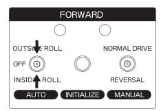
Make sure the AUTO switch for the Feed unit is OFF.
