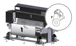
Pass the roll media through over the roller in the front, then under the roller in the back as shown.
