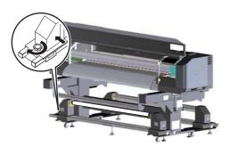
Tighten the handle on the non-origin side of the front roll unit.
