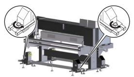
Loosen both handles on the rear roll unit.
