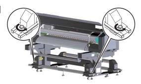
Loosen both handles on the front roll unit.
