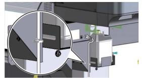
Pass the power cord through the clamp on the lower side.
