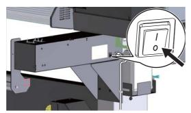
Press the power button to turn the power OFF.
