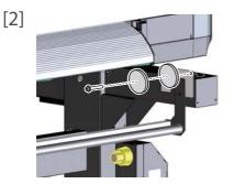
Attach the weight (2 pieces) to the counter weight mount board with a M4 $\times$ 30 screw.
