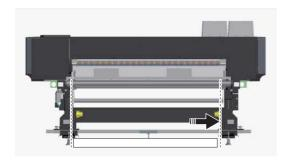
Move the non-origin side of the rear roll unit to the appropriate position so that the roll media can be attached to the unit.
