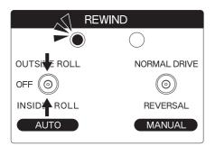
Set the AUTO switch on the side where the red lamp blinking to "OFF".
