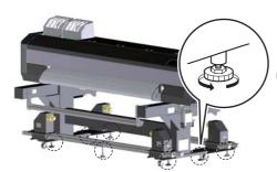
Rotate all the leveling adjusters on the stand (x4) and take-up unit (x4) anticlockwise to raise them.
