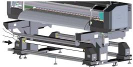
Move the non-origin side of the front roll unit and attach the paper core.
