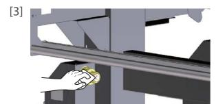
Using a soft cloth dampened with water and wrung it out, clean off paper dust from the media flanges on both front and rear rail unit.
