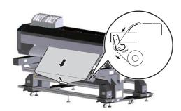
Fix the leading edge of the media using tape so that the tip is parallel to the paper core.
