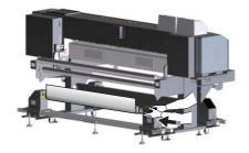
Move the non-origin side of the rear roll unit and attach the roll media.
